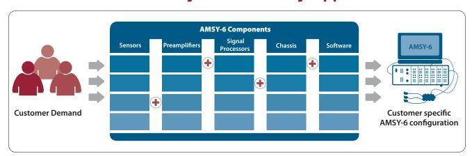
The Vallen AMSY-6 system covers the entire AE measurement chain. Using modular components customized and expandable systems are configured, comprising sensors, preamplifiers, signal processors, system chassis, PC interface
