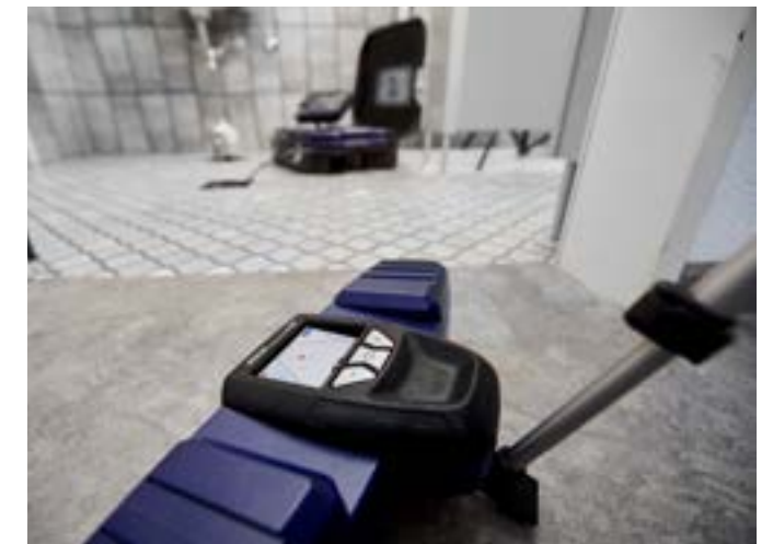
Precise location of the camera head with the Wohler L 200 Locator.
