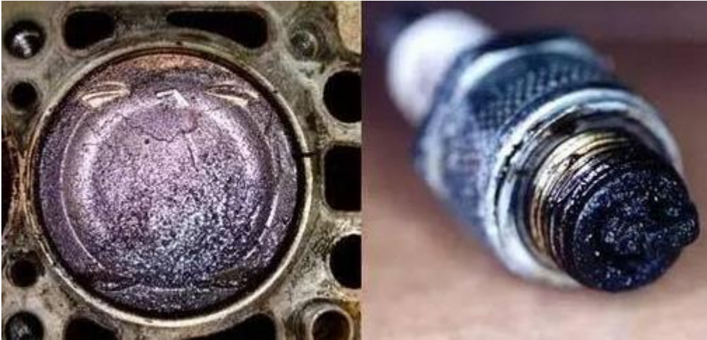
Piston and spark plug carbon
