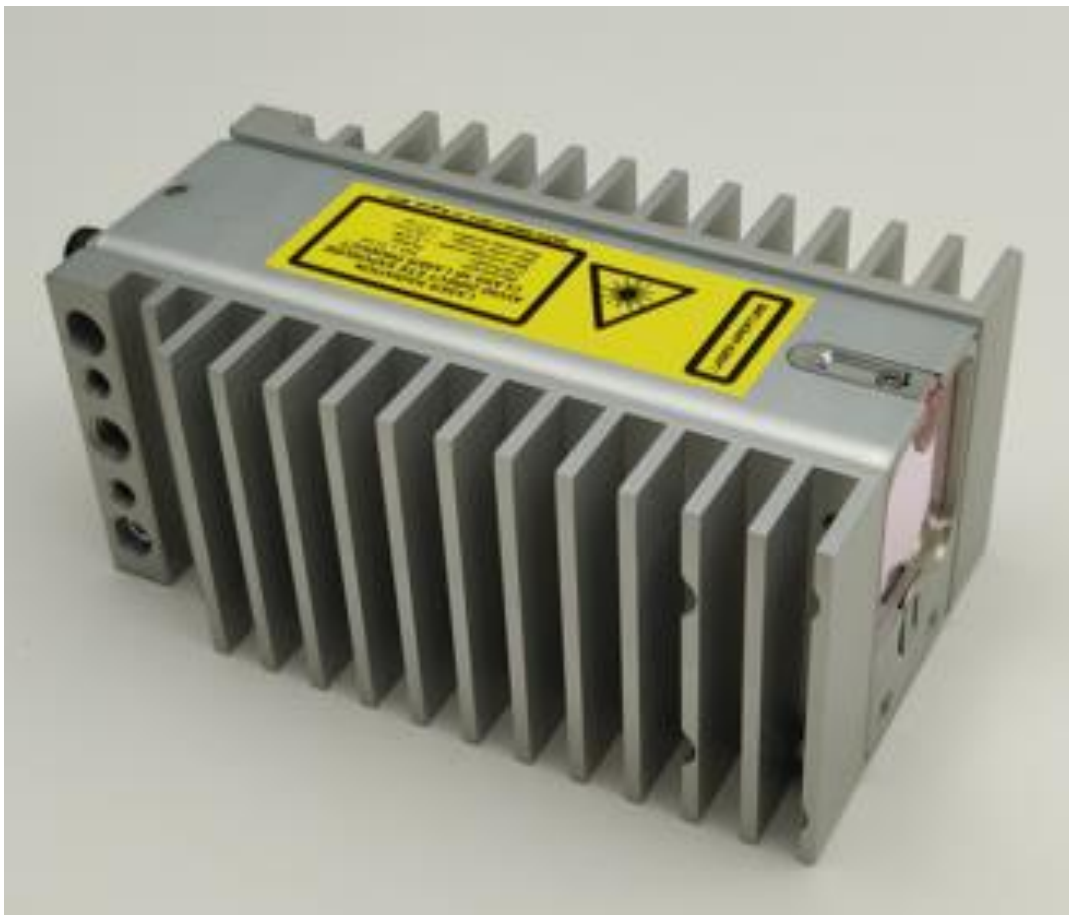
Fig. 2.9. Heat sinks successfully mounted.
