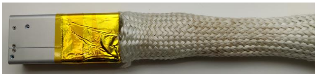
Fig. 3.6. Thermosleeve B pulled over the cables and hoses.
