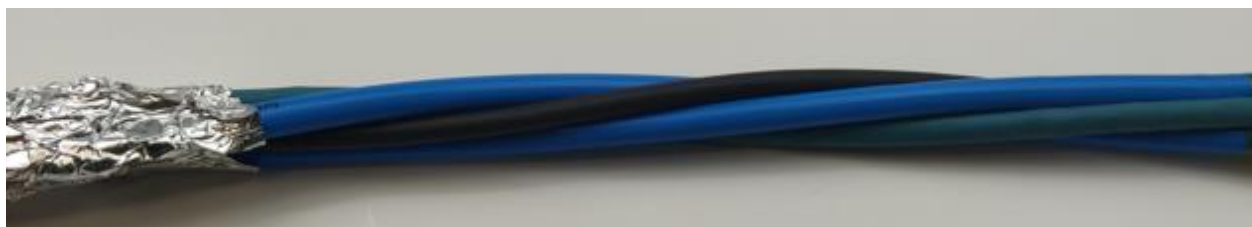
Fig. 3.2. Twisting the cooling hoses around the electrical cables.
