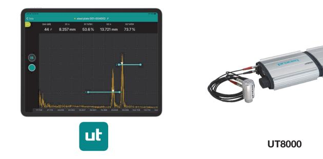
Flaw detection of metal and composite components using ultrasonic testing
