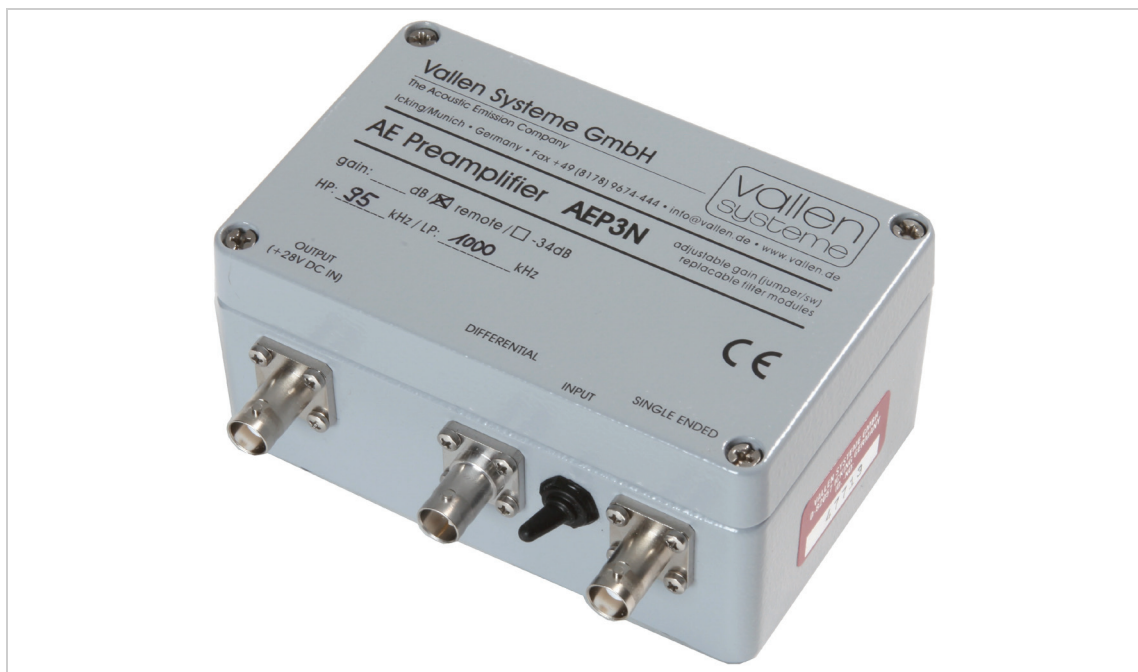
Figure 2: AEP3N preamplifier. Connectors from left to right are: (i) signal output and power supply input, (ii) differential BNC input and (iii) single ended BNC input.
