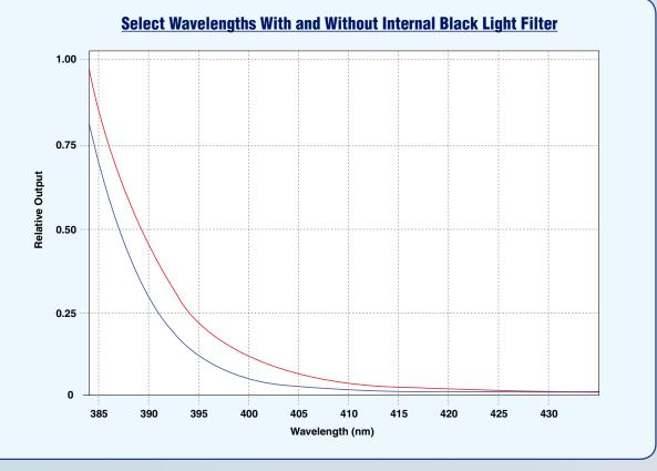
As the wavelength of the OPTI-LUX<sup>™</sup> 365 moves into the visible light range, the black light filter significantly reduces the UV-A output of the lamp by as much as 50% at 400 nm. OPTI-LUX™ 365 flashlight with BF-365LX external black light filter accessory
