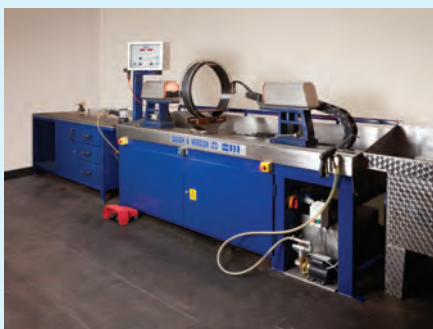
MAGAZON EBU MPI Benches ideal for testing large components
