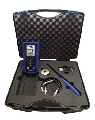
Baugh & Weedon is pleased to present the LumaFlux, a truly Innovative NDT Product. The LumaFlux is a combined Dual UV / White Light Meter and Tangential Field Strength Meter in one rugged Instrumentation package.
