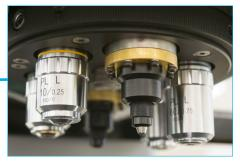
The turret can be configured with either 1 or 2 indentor actuators, and combined with a maximum of 4 objectives. The second indentor can be added after installation.
