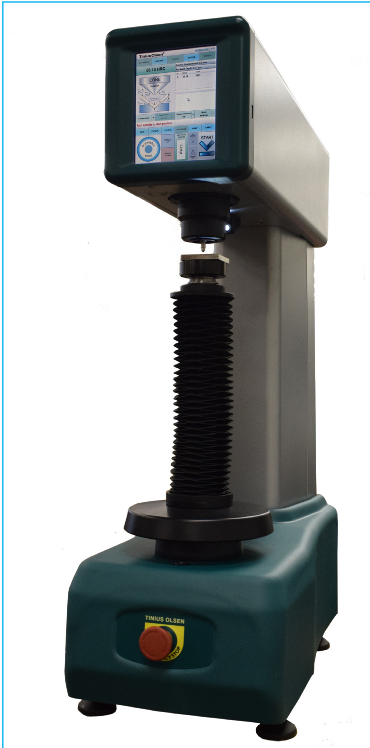
Fig. 1. Model FH-1-4 Rockwell/Superficial Rockwell hardness tester.
