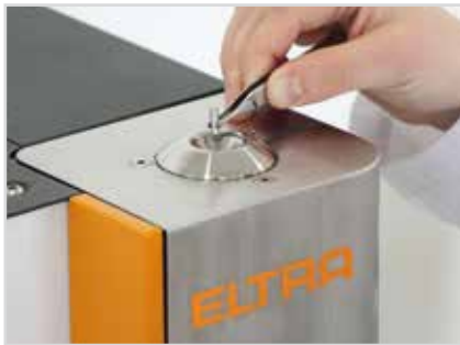
Manual sample feed to the sample port system
