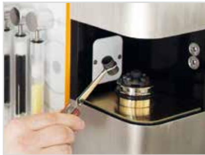
Placing a crucible on the lower electrode
