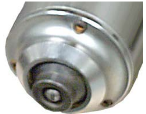
Shown: Indenter with shroud assembly. The indenter is a 10mm tungsten carbide ball welded to a threaded shaft.
