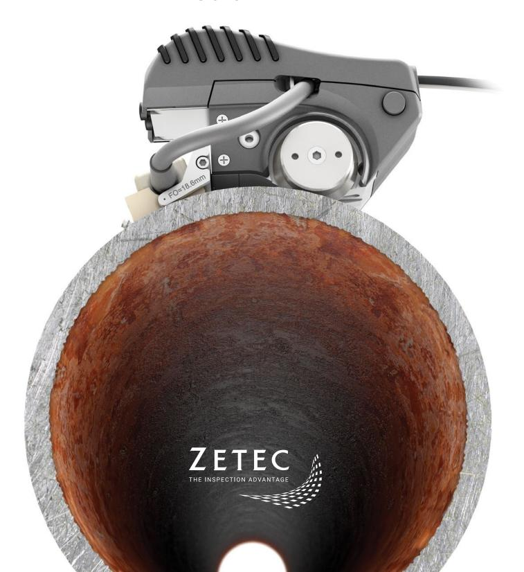
NDT PAINTBRUSH, BY ZETEC. AN EVOLUTION IN THE FIELD OF INSPECTION SOLUTIONS FOR THE DETECTION OF WALL-THICKNESS REDUCTIONS DUE TO CORROSION, ABRASION OR EROSION. THANKS TO NDT PAINTBRUSH, YOU CAN MAKE THE RIGHT DECISIONS AND LEAVE UNCERTAINTY BEHIND.
