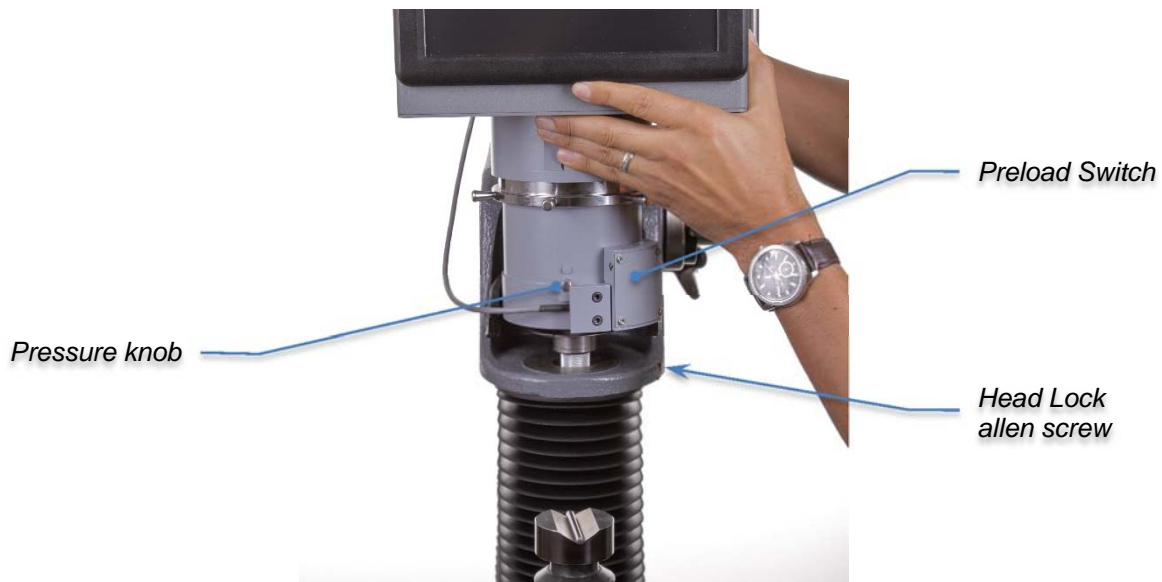
Installing the Test Head
