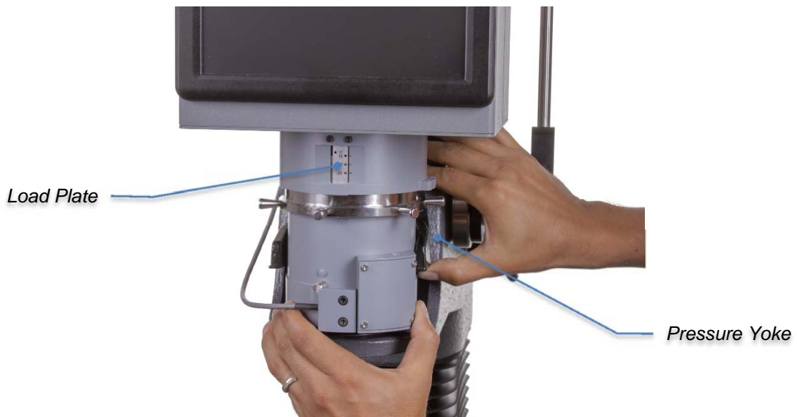
Installing the Test Head
