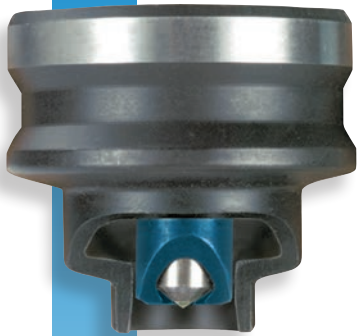
Indenter and standard shroud (in false color) shown in normal operating position with the standard clamping shield
