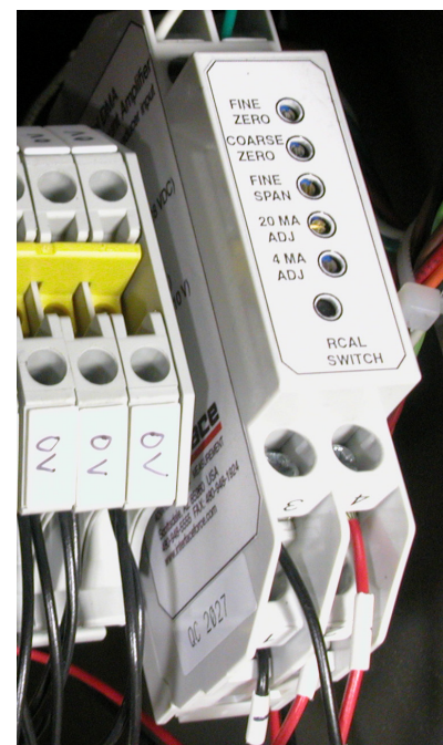
"Fine Span" control. located on the amplifier inside the right side panel.
