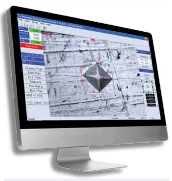
C.A.M.S. provides **real time SPC**, including XBar-R chart, chronological test result history with date and time "stamp", histogram, average, standard deviation and Cpk.
