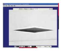
Achieving good accuracy and repeatability are more complex than simply obtaining good results on perfectly produced test blocks using a technician at a heightened level of attention. The C.A.M.S. system can operate exceptionally well on a variety of test surface conditions, and with the range of surface leveling and rounding at the edge of a sample, that is typically encountered on mounted test samples.
