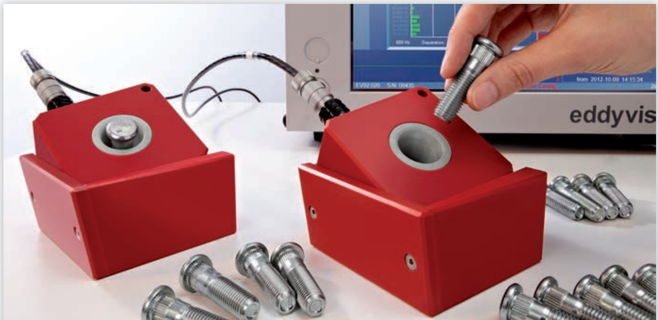
Fixture for manual eddy current structure test in the lab.
