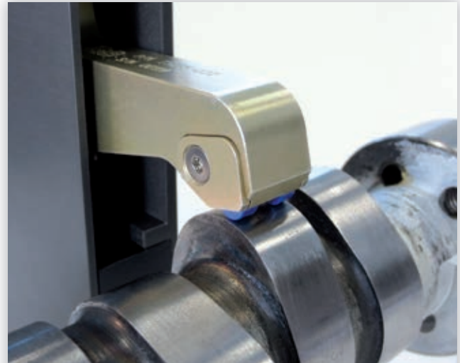
Crack detection probe box for contacting testing on eccentric parts like camshaft lobes for cracks and grinder burn; large diameter range is covered; up to 300 rpm (depending of part geometry), ceramic supports for long life-time. Solutions for structure test on camshafts on request.
