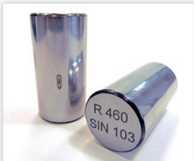
ibg crack and grinder burn master with EDM cracks and pores for simulation of surface open defects and with laser defects for simulation of grinder burn; intensity mere residual stress (cutting far left) and beginning annealing zone (left).
