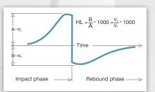
Velocities are measured using a permanent magnet in the impact body that generates an induction voltage in the coil which is precisely positioned in the impact device. The detected voltage is proportional to the velocity of the impact body. Signal processing is then providing the hardness reading.
