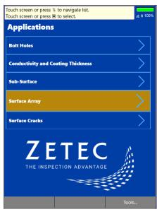
Once the MIZ-21C is fully powered up, the initial display will show the various application types supported by the MIZ-21C. The MIZ-21C organizes techniques under application categories to quickly identify the best technique for inspection requirements. Select the category to view avilable techniques currently loaded.
