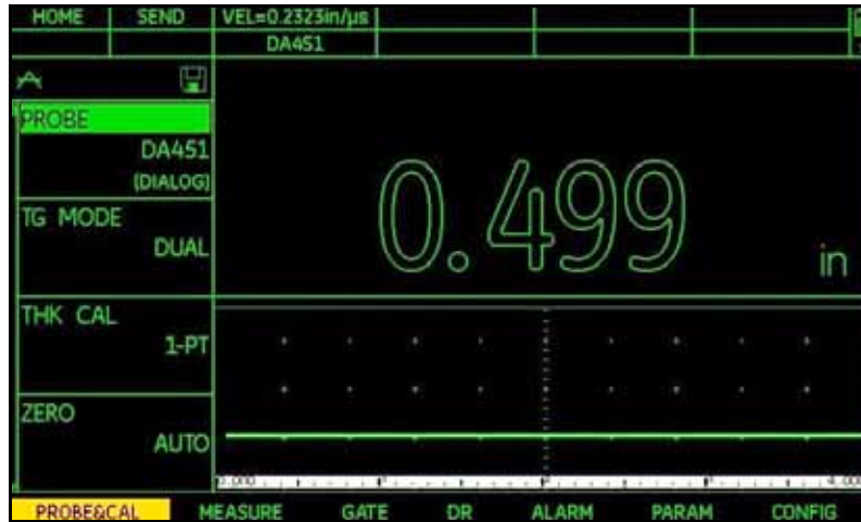
Figure 20: Display for Connected Dialog Probe (Dialog Indicated by Signal at Bottom)
