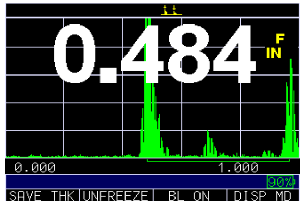
ECHO 9W – Includes Waveform, Coating Thickness
