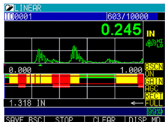
ECHO 9DLW – Includes Waveform, Datalogger, B-scan, Coating Thickness, Temperature Correction
